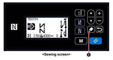
On the sewing screen which is displayed in the case free stitching, constant-dimension sewing or multi-layer stitching is selected, press **5** to display the sewing pattern edit screen.
