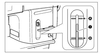
Confirm that the top of oil amount indicating rod **1** is between the upper engraved marker line **2** and the lower engraved marker line **3** of the oil amount indicating window. (For the details, refer to "2-14. Lubrication" p. 12.)
