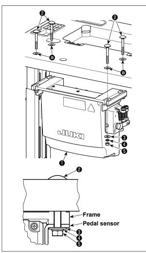
Install control box ① on the table using four holes
