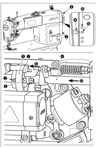
Turn thread trimming cam ③ in the direction of arrow until the outer periphery of thread trimming cam groove ⑤ comes in contact with roller ② and stops. At this position, fix thread trimming cam setscrew ⑦.
