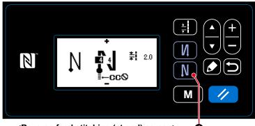
A held pressed for one sec-Keep ond. The reverse feed stitching (at end) edit screen is displayed.
