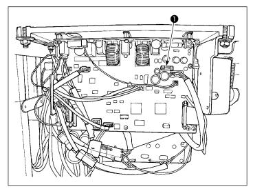
The machine uses the following one fuse : MAIN PWB
