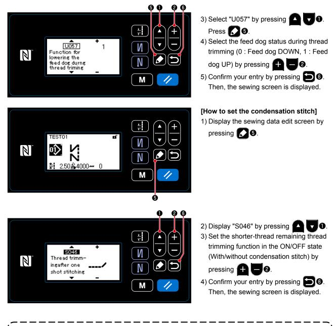
The condensation operation should be turned OFF before thread trimming is performed at a position where there is no material since thread loop formation at the time of thread trimming becomes unstable.
