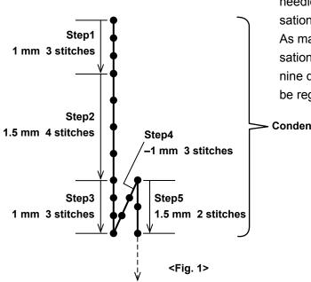
Condensation stitches can be sewn while specifying needle entry points as desired, by setting a condensation custom.
