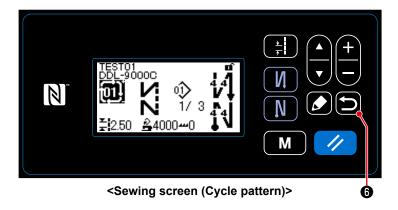
Press **D (b)** to confirm the data and return the current screen to the sewing screen of the edited cycle pattern.
