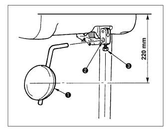
Insert knee lifter pad **1** into attaching hole **2** and tighten it with bolt **3**.
