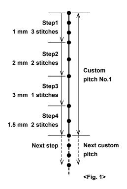
It is possible to register as many as 20 different sewing designs each of which consists of several different pitches (10 steps at the maximum).
