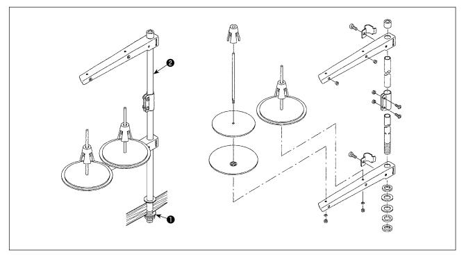
1) Assemble the thread stand unit, and insert it in the hole in the machine table.
