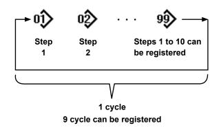
It is possible to combine several different sewing patterns as one cycle pattern for sewing. As many as 10 patterns can be input in one cycle pattern. This function is helpful in the case several different patterns are regularly repeated in a product sewing process.
