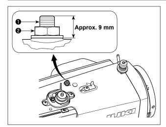
When sewing velvet or the like which is fluffy, slippage of material or damage of material is reduced by using screw **1** for presser foot micro-lifting. Lower the presser foot and set the state that the feed dog is lower than the throat plate.
