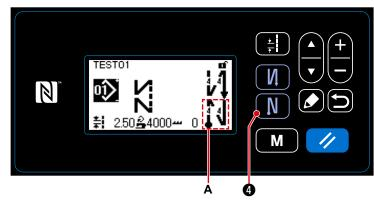
When pictograph **A** is displayed on the screen, reverse feed stitching (at end) is enabled.
