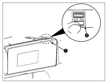
USB thumb drive insertion position The USB connector is provided on top ① of the operation panel.
