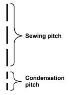
In the case of carrying out shorter-thread remaining thread trimming (when condensation is placed in ON), set values of the condensation pitch and the number of stitches are adjustable. Adjust those set values appropriately according to the item to be sewn.
