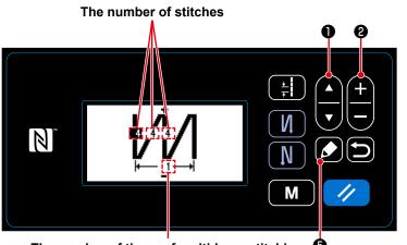
The number of times of multi-layer stitching Multi-layer stitching pattern edit screen>  When a multi-layer stitching pattern is selected, the multi-layer stitching pattern edit screen is displayed by
