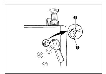
By means of the thread tension release releasing mechanism, sewing can be performed without slackening the needle thread tension even when the presser foot is lifted during sewing. (Even when the presser foot is slightly lifted at the
