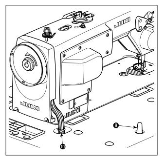
4) Securely attach head support rod **9** to the table until it goes no further.
