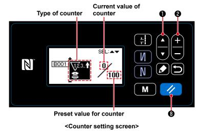
The counter setting screen is displayed to enable setting of data on the counter.
