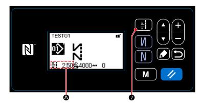
Stitch length is displayed in section (2) on the panel. (Example of display : 2.50 mm)
