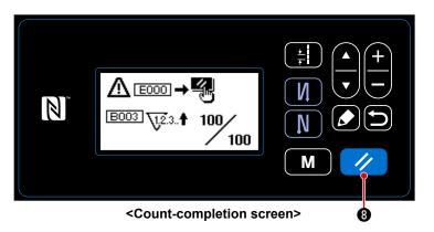
When the predetermined conditions are satisfied during sewing, the count-completion screen is displayed.
