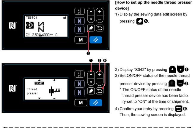
In the case the memory switch "U056 Reverse-rotation needle-up after thread trimming" is enabled, the length of needle thread becomes longer. So, in this case, the needle thread presser device should be set to "OFF".
