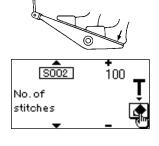
After the completion of sewing steps (the last stitch), depress the back part of pedal. Then, the data entered for the current step under the teaching mode is confirmed and the screen is changed to the teaching screen for the next step.
