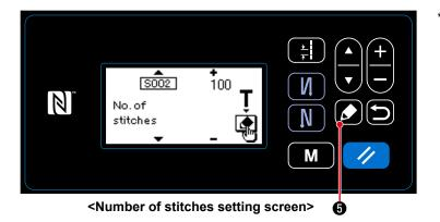
In the case the constant-dimension sewing pattern is selected, the teaching screen is displayed by pressing for the number of stitches. (Only in the case the number
