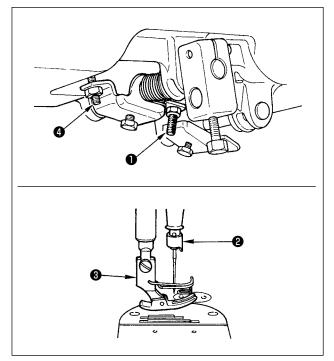
The standard height of the presser foot lifted using the knee lifter is 10 mm.
