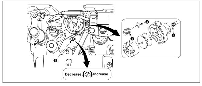
Tighten (turn clockwise) oil amount adjustment screw **1** to increase the amount of oil in the hook, or loosen (turn counterclockwise) to decrease it.
