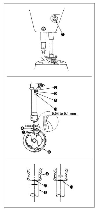
Adjust the timing between the needle and the hook as follows :
