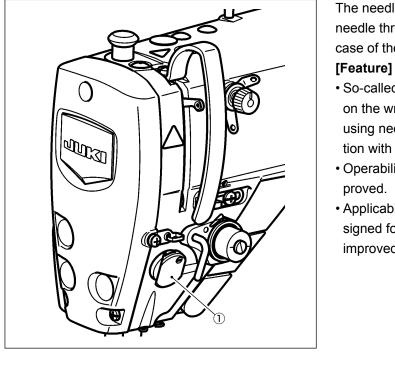
The needle thread presser device is able to tuck the needle thread on the wrong side of material as in the case of the conventional wiper device.
