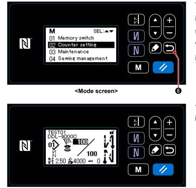
The data on the counter function entered is confirmed by pressing **(b) (c)**. Then, the screen is returned to the mode screen. With another press on **(b) (c)**, the screen is returned to the sewing screen.
