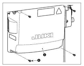
3) Install control box cover 3 with four setscrews 4.
