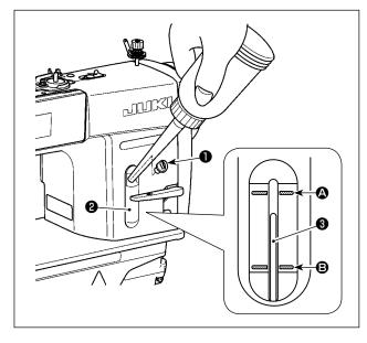
Fill the oil tank with oil for hook lubrication before operating the sewing machine.
