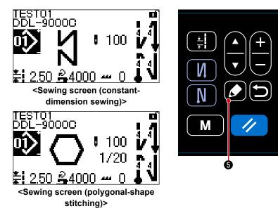
The sewing pattern edit screen is displayed by pressing **5** on the sewing screen.
