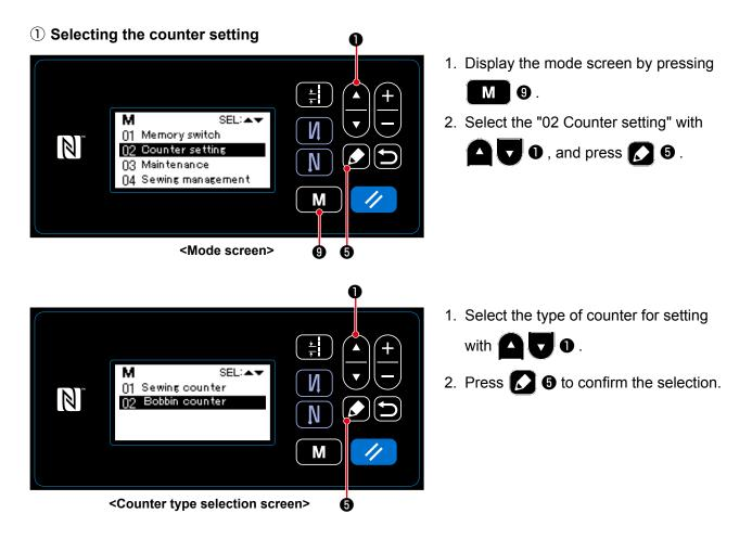
2 Setting the type of counter, current value of counter and preset value for counter
