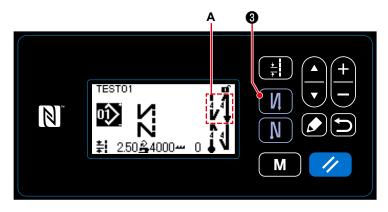
In the state pictograph **A** is displayed on the screen, the reverse feed stitching (at start) is enabled.
