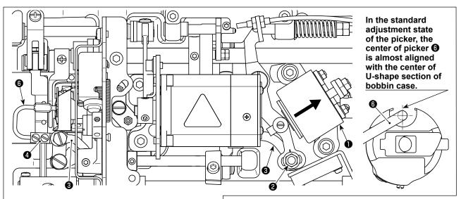
Once the standard adjustment is carried out correctly, there is a slot-shape space in picker link () to allow the picker to make a necessary returning action (damper function).
