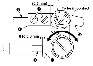
The picker device is used in order to stabilize idling of the bobbin at the time of thread trimming.
