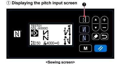
Press () on the sewing screen to display the pitch input screen.
