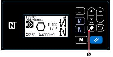
① Displaying the polygonal-shape stitching pattern edit screen
